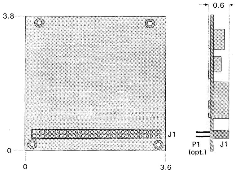
Figure 1. Basic Mechanical Dimensions (8-bit Version)
