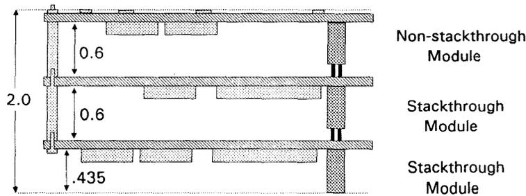
Figure 2. Standalone Module Stacks
