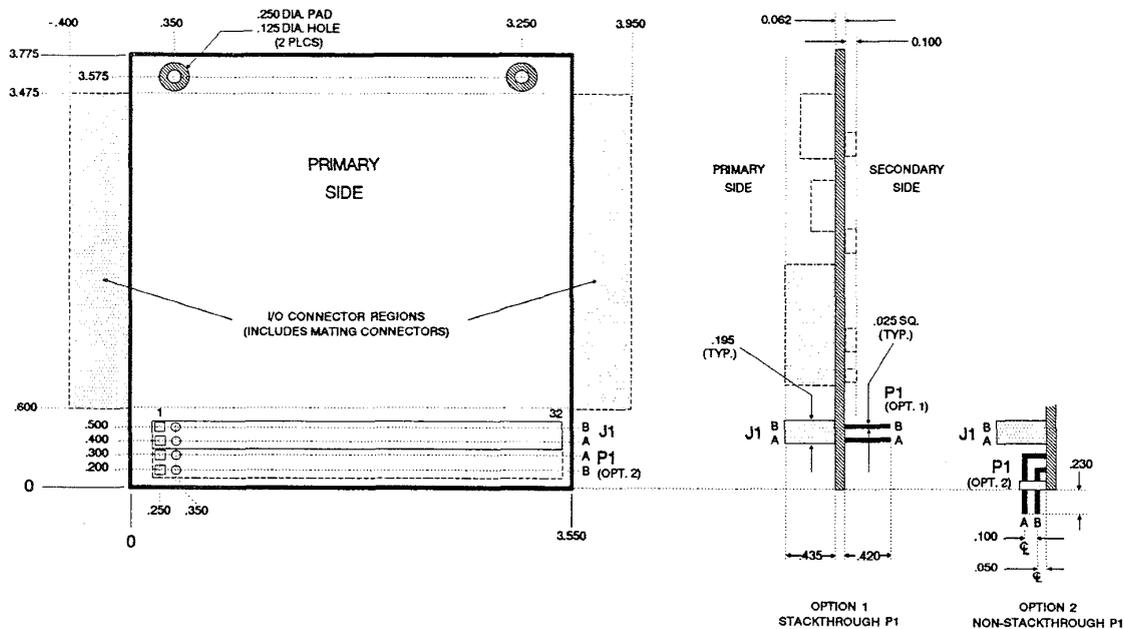
Figure 4. Detailed Mechanical Dimensions (8-bit Version)
