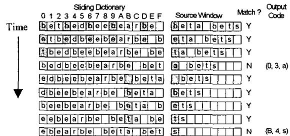
Figure 5. Operation Principle of LZ Compressor [12]
