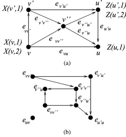
Fig. 4. (a) Network with two source and two sink nodes. (b) Corresponding labeled line graph. Labels in (b) are omitted for clarity. The edge  $e_{vu}$  does not feed into any other edge and no edge feeds into  $e_{vu}$ , which renders an isolated vertex in the labeled line graph.
